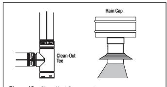
Figure 48 - Clean Vent Components
